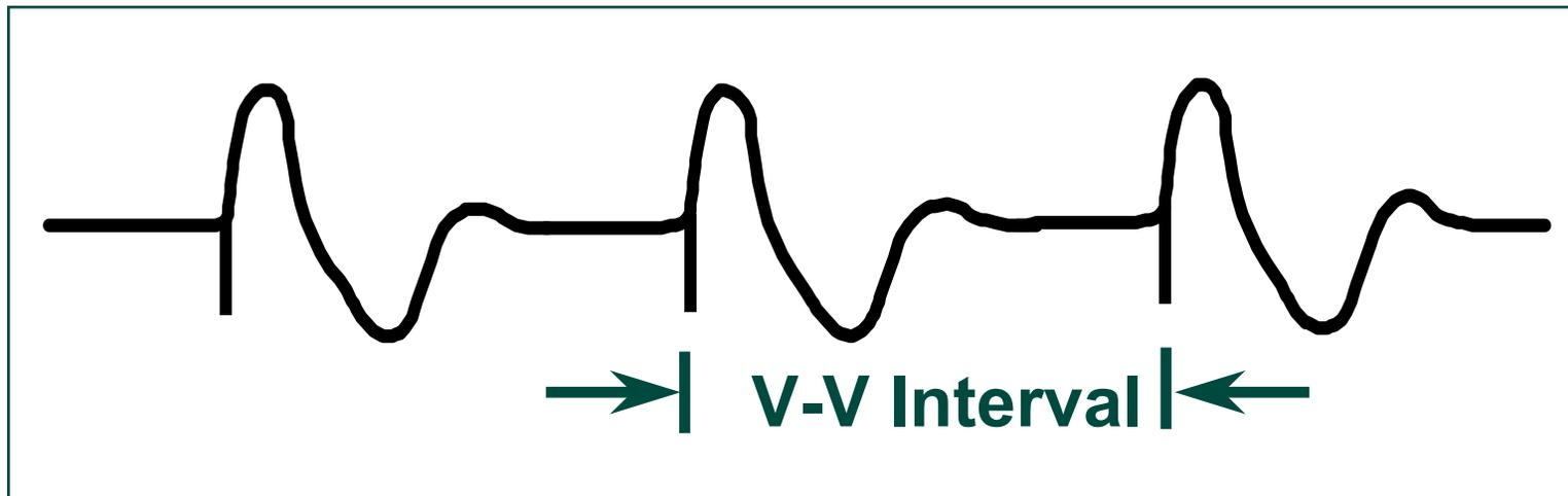
$$\text{Interval (ms)} = 60,000 / \text{rate (ppm)}$$
