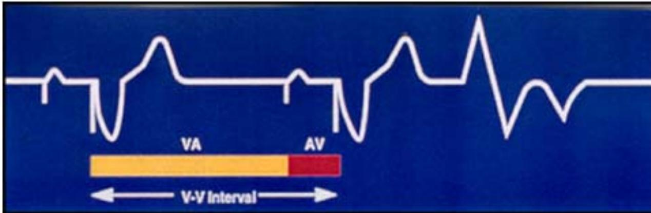
**Atrial-Based Timing: Atrial events start timing cycles**
